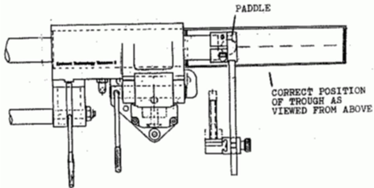
The paddle is threaded into the counterweight clamp and can be raised or lowered by rotation. Turn the paddle until it is positioned about 1/16" above the dry trough across the full travel of the tonearm. (It is OK to move the air bearing back and forth without the air pump operating.)
