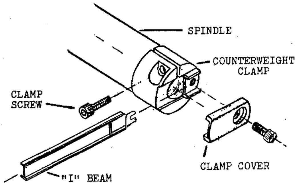
In order to install the kit you must first remove the counterweight assembly from the backside of the air bearing spindle. This is done by loosening the top screw on the counterweight clamp. Loosen this screw about one full turn and pull the clamp off of the end of the spindle. Do not overtorque these screws when re-assembling this part. The 3/32" allen wrench which is supplied with the ET-2 is the only tool required for installation.
